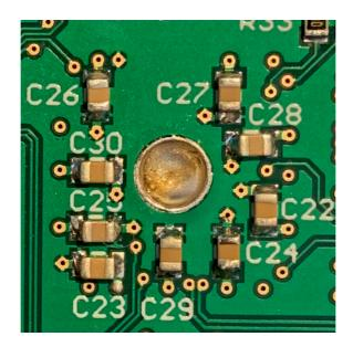
flux here and flood solder into the via. Heat will tend to flow into the internal planes of the PCB so use a hot iron and beware of forming a 'cold' solder joint. When complete it should look something like this :-
