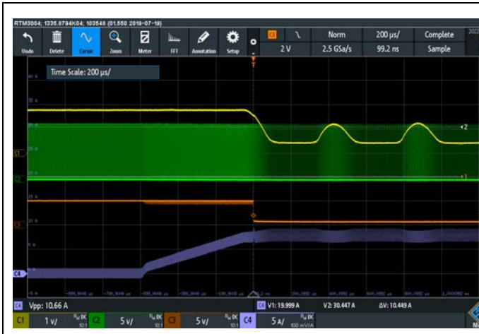
Figure 21 OCP for Clamp mode CH1: VOUT CH2: SW CH3: PG CH4: IL
