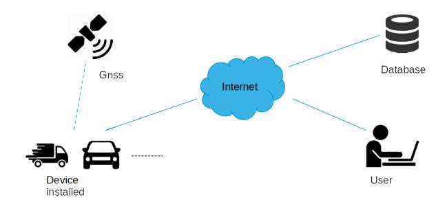
The diagram shows a typical use of the product: a user configures the device to receive information. The device is installed on various devices (cars, motorcycles, trucks, or any other place you want to monitor). The device communicates with the satellites to receive satellite information and depending on how it is configured it can send information to a specific terminal or data to a database via the GSM/LTE module.
