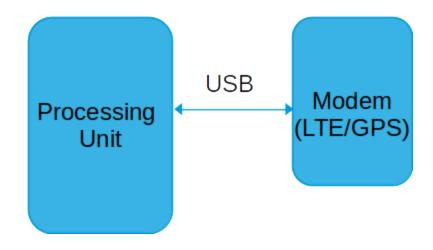
The models of the Processing unit and the GNSS/LTE module are shown below. The two modules are connected via USB.
