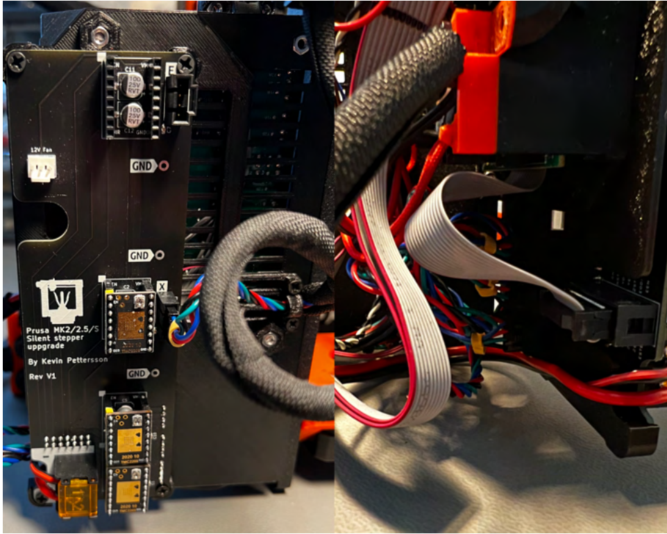
Figure 10: View of front and back of XYZE upgrade board for X, Y and Z installation, NOTE depicted image is of V1, V1.1 looks slightly different.
