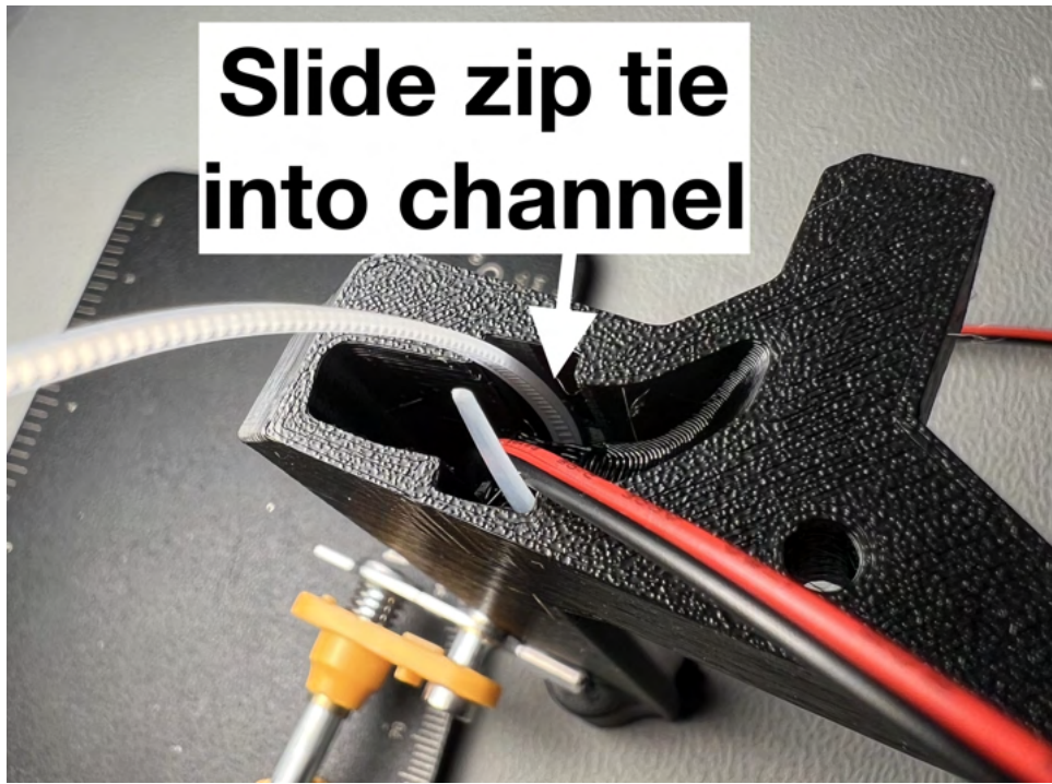
Figure 13: Strain relief installed on light holder.
