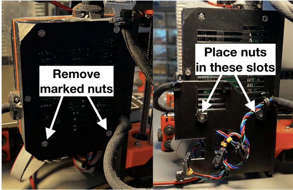
Figure 8: Rambo base, without and with the upgrade board holder-
