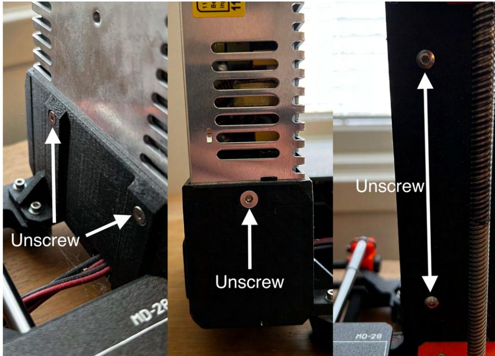
Figure 2: PSU mounting screws.
