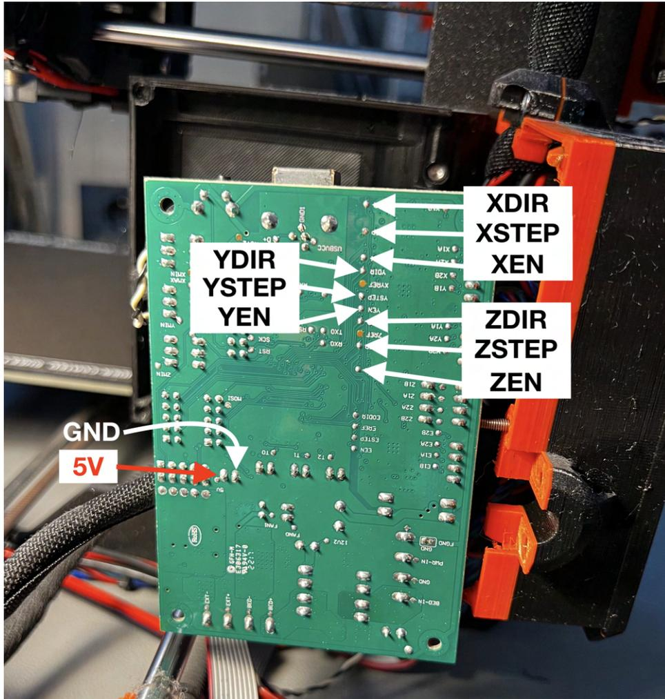
Figure 6: Recommended position for Rambo control board to solder data pins.
