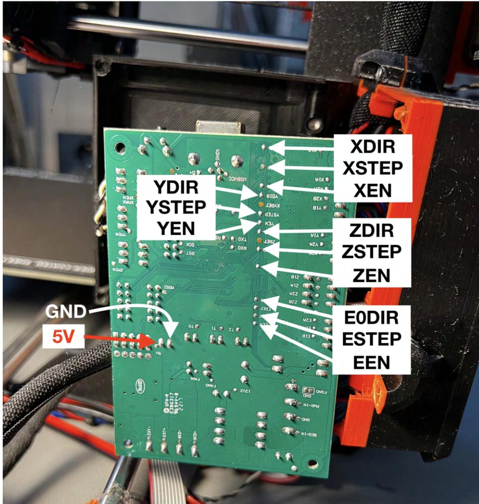
Figure 10: Recommended position for Rambo control board to solder data pins.
