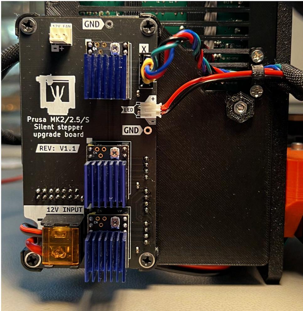
Figure 9: View of front of upgrade board for X, Y and Z installation, with the optional X-axis LED light.
