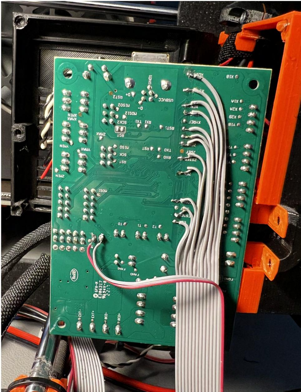
Figure 11: Data pins soldered to Rambo for **XYZE** board.
