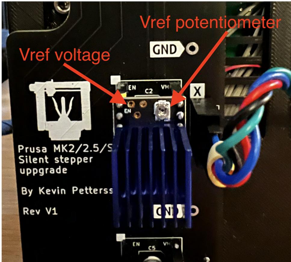
Figure 18: Vref potentiometer and measuring point illustrated on a TMC2209.
