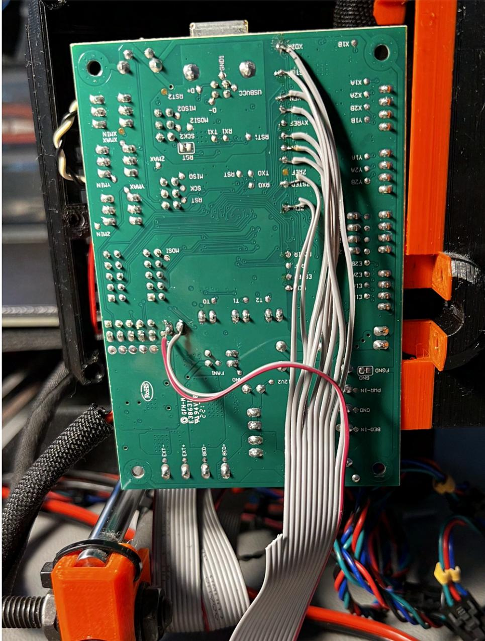
Figure 7: Data pins soldered to Rambo, pins 12, 13 and 14 left floating in this installation of a XYZ board.
