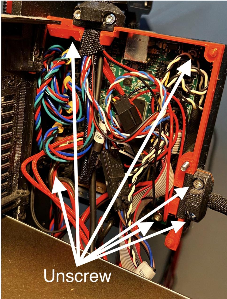
Figure 5: Front side Rambo control board.
