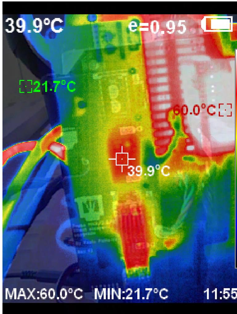
Figure 19: Thermal image of TMC2209's and X axis stepper motor 2 hours into a 4 hour PETG print.
