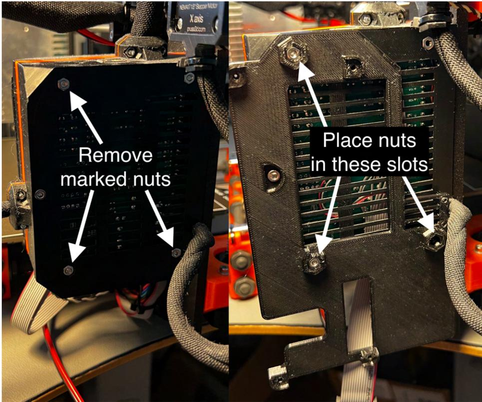
Figure 12: Rambo base, without and with the upgrade board holder-
