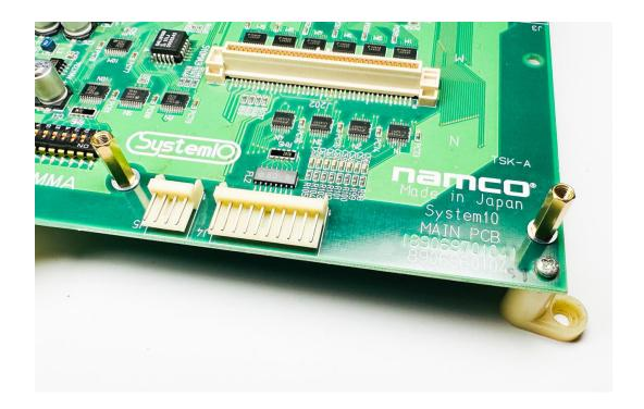
3. Using the 2 remaining screws, mount the stereo board to the brass standoffs.
