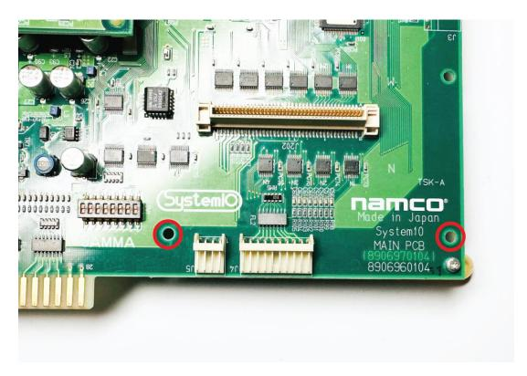
2. Place a washer on one of the screws and insert it through one of the mounting holes from the bottom of the Namco System 10 PCB. Place a second washer on the screw from the top of the PCB then screw one of the brass hex standoffs on to the screw. Repeat the same process for the other mounting hole.
