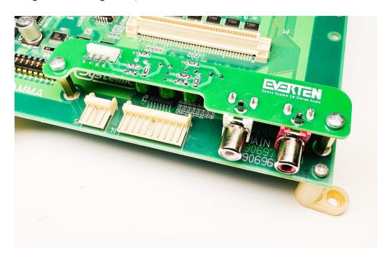
${\bf 4.} \quad {\bf Connect\ the\ wire\ harness\ to\ the\ Namco\ System\ 10\ PCB\ firs,\ then\ the\ stereo\ board.}$
