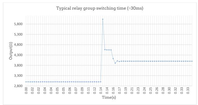
Above: Typical relay group switching time. The example is monitoring the process of switching from  $3k\Omega$  to  $4k\Omega$ , with the measurement mode 2-wire and the configuration NPLC=0.05.
