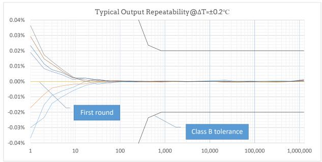
Definition:  $\Delta T$  = ambient temperature at test – Tcal
