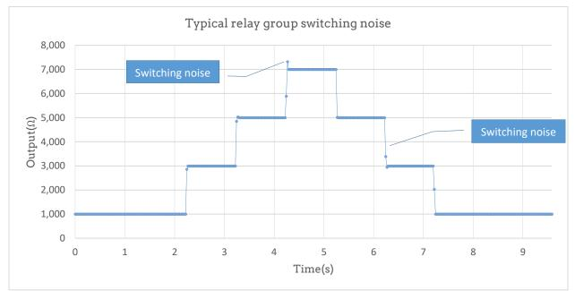
Above: The "output resistance noise" generated by relay switching occurs on the rising or falling edge, and is more obvious during some resistance switching. It should be noted that the relay switching algorithm of the QR10 is not specifically optimized, so in some cases, the output may be open or shorted for a short period (ms level).
