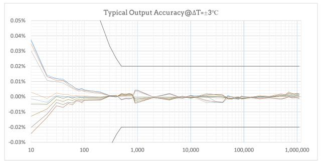
Above: Accuracy is based on 10 consecutive rounds of testing of the same sample in a thermostat (temperature variation range: Tcal-3°C to Tcal+3°C). Errors are based on direct comparisons with reference meter readings and do not include the uncertainty of the reference meter itself.
