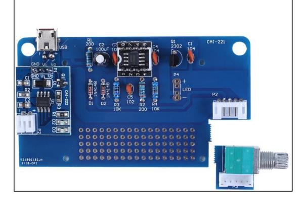
Step 18: Identify the positive(anode) and negative(cathode) lead of LED. The leads of the LED must be installed correctly, otherwise the LED cannot be turned on. Here are four methods as following:
