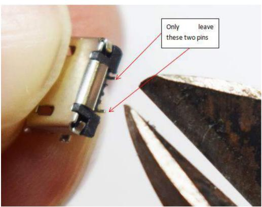
Solder the micro usb socket in place following the image, if you do not want to use the micro usb socket to power your Christmas tree, then you can use the 5V power supply pads. The polarity is marked on the board.
