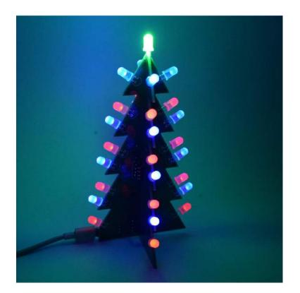
Next, we want to use the pin to connect the three PCB into a three-dimensional shape tree, first solder the shorter pin to one of the small parts of the tree.
