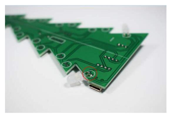
Solder all the LEDs on both sides of the tree. Remember to adjust the position and angle of the LED to make sure all are more or less similar. This is how it should look like!
