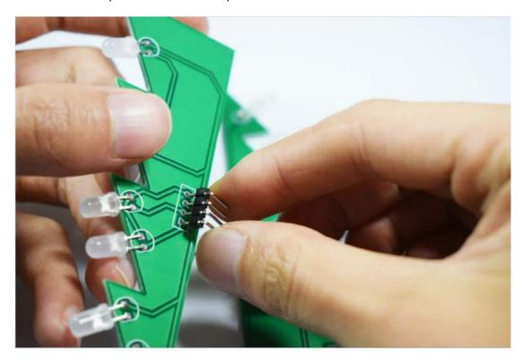
Then, insert the other part of the legs in the main board. Adjust the position before soldering all the legs.
