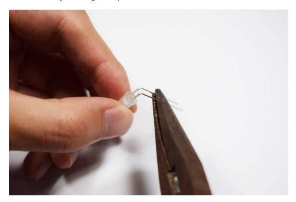
Then insert the LED long leg corresponding to the square pad, remember not to solder the LED in the wrong direction!
