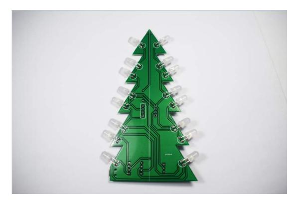
Then solder the tip of the LED tree, the soldering method is the same as before:
