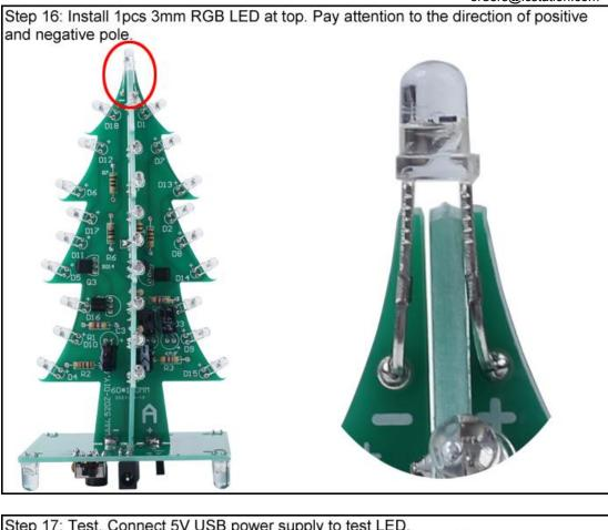
Step 17: Test. Connect 5V USB power supply to test LED. It is OK if all LED flash automatically after turning on the power switch.
