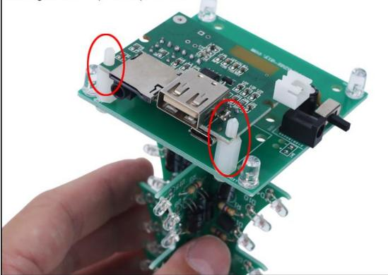
Step 20: Fix 2pcs M3\*8mm Nylon Column on M3\*10+6mm Nylon Column Screw. Be careful not to be too tight.
