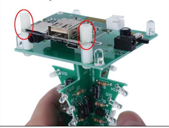
Step 21: Fix 2pcs M3\*20mm Nylon Column on PCB-C by 2pcs M3\*6mm Nylon Screw.
