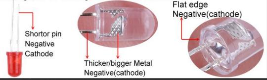
Step 14: Install 10pcs 3mm Blue LED at D1-D10. Pay attention to distinguish between positive and negative pole.
