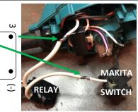
(Leave switch in on position for normal operation) CAUTION!! 120v/240v UNPLUG FROM ROUTER FROM POWER SOURCE BEFORE CONNECTING! IF YOU''RE NOT COMFORTABLE DOING THIS...DON'T!
