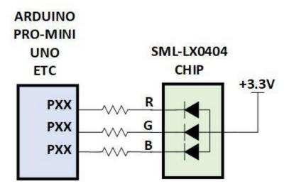
The SML-LX0404 chip is a current sink and can be connected to any MCU. The anode should be connected to +3.3V. The reason for this is the Series resistors are calculated for current limiting based on +3.3V. Changing the anode voltage to another source will change the brightness emitting from each LED. Because the SML-LX0404 chips are current sink, the user can connect to either +5V or +3.3V Arduino (or other MCUs) and control each LED.
