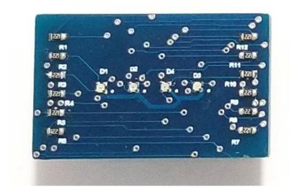
The top down view is shown below. The LEDs are located on the top and organized as D1 through D4. The connectors are shown as looking through the board.
