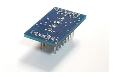
The EPT-SML-LX04-LD-X2 is a breakout board that includes four LED RGBs. This Board provides a simple interface to control four LED RGBs for a total of 12 LEDs from any MCU (including the Arduino family). It is designed to connect directly to the standard bread board with a reduced footprint. Once connected to an MCU, the MCU can provide a sink for each LED.
