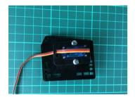
Pass the servo motor through the sleeve and mount the cable to the side plate with 8mm screws as before.
