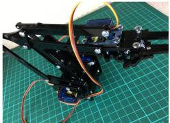
Now that we have completed the robot arm part, we place our robot arm on our servo motor, which will enable the robot arm on our vehicle to turn left and right.
