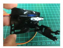
You should see the shoulder slot in part 7 (front brace). Insert the shoulder into the slot, then insert the base piece into the slots on the left assembly and lift upward to engage the slots in the shoulder.
