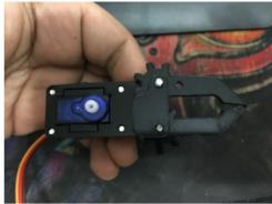
Attach a servo motor end to part 30 and secure it to the servo motor using a machine screw. Attach part 29 to part 30 using two 6 mm screws.
