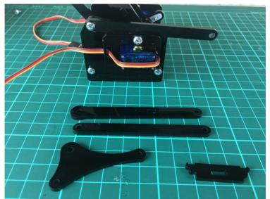
Attach triangle 19 to part 31 and part 13 with a 10mm screw. Do not over tighten as we need all these parts so that we can move freely.
