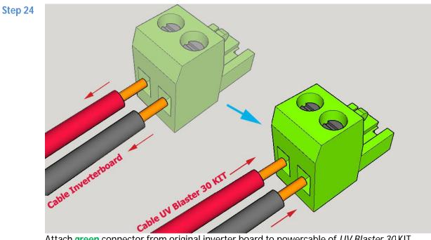
Attach green connector from original inverter board to powercable of *UV Blaster 30* KIT **NOTE** : The green socket at the motherboard, text "-LED+" is printed and indicates the position of **plus** (red cable) and **minus** (black cable).
