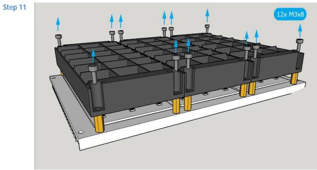
Remove 12 screws which fixate black distance-beds at metal spacers from heatsink.
