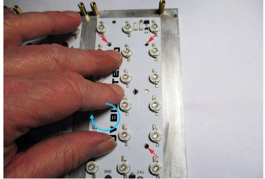
Slightly swirl / rotate UV Blaster 30 boards and push gently to smear out the thermal grease. Next, align UV blaster 30 boards with holes at heatsink.
