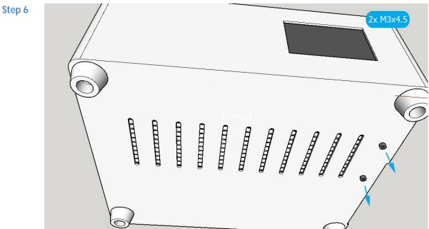
Remove 2 screws of inverter-bracket at bottom of case **NOTE** : Make sure you keep the inverter-bracket inside the case stable, with 1 hand
