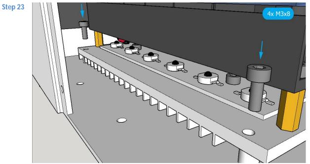
Align heatsink and insert 4 screws back, in all 4 corners of heatsink, to fixate it to case
