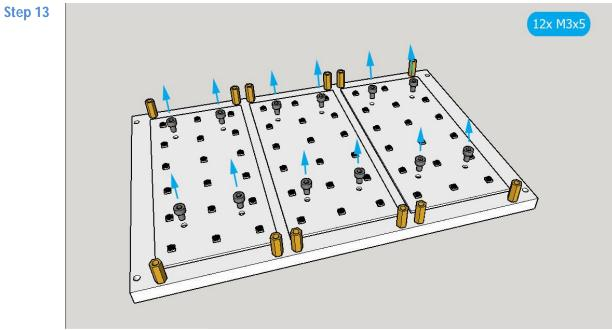
Remove 12 screws, which fixate UV boards to heatsink
