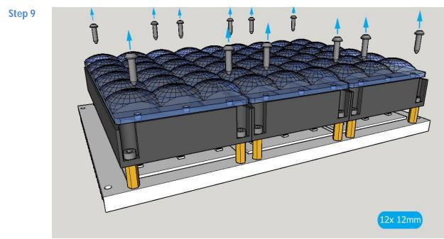
Remove 12 screws which fix 3 LED-lenses to black distance-beds.
