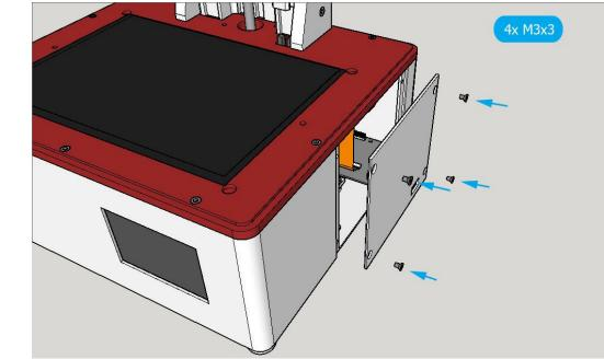
Align USB-panel back to original position at side of case. Insert 4 screws to fixate USB side-panel. **NOTE** : The USB-connector needs to be be easy accesible.
