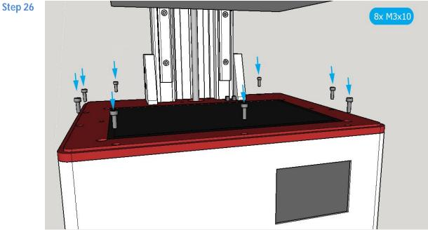
Align red top-plate back onto case and insert 8 screws to fixate it.
