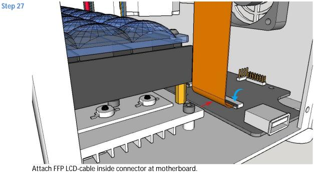
Attach FFP LCD-cable inside connector at motherboard. Carefully flip black plastic lid (75° angle) from FFP-connector down to fixate FFP LCD-cable
