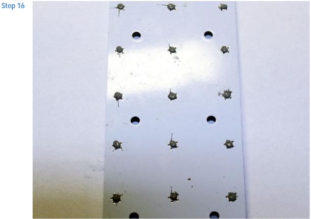
Make sure the complete board is perfectly flat, even at the corners. Apply thermal grease at backside of each *UV Blaster 30* board, also at the corners. Suggestion : Add a tiny dot where a LED is located (indicators : tiny thermal support-holes).
