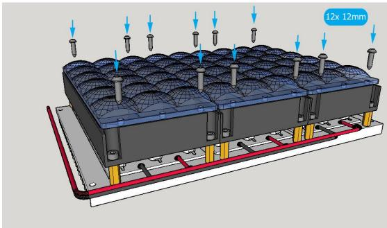
Insert all 12 screws back to fixate LED-lenses **IMPORTANT NOTE :** Don't tighten the screws too much or it may irreversable damage the transparant plastic LED-lenses. Suggestion : Clean top of LED-lenses with microfiber cloth.
