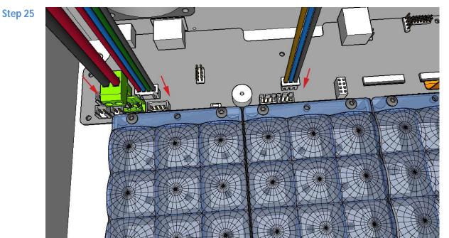
Attach white connector with 3-cables to "*Z*-" sensor (brown, blue and black) Attach white connector with 4-cables to steppermotor (red, blue, green, black) Attach green connector with 2-cables to *UV blaster 30* KIT (black and red)
