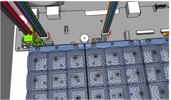
Detach white connector with 3-cables to "*Z*-" sensor (brown, blue and black) Detach white connector with 4-cables to steppermotor (red, blue, green, black) Detach green connector with 2-cables to inverter board (black and red) **NOTE** : This green connector is needed (later) for the *UV Blaster 30* KIT
