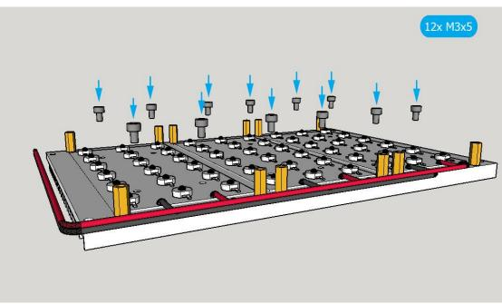
Mount 12 screws back into heatsink to fixate UV Blaster 30 boards
