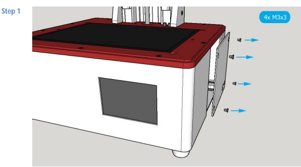
Remove 4 screws from USB side-panel and remove panel **NOTE** : USB side-panel can be fixed to red top-plate with a piece of tape
