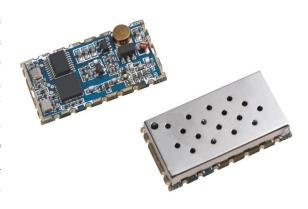
There are two frequency bands of SA818: SA818-U and SA818-V. The only difference is the frequency range. The others are same, including module size, interface, software protocol, etc. The two modules' frequency ranges are:
