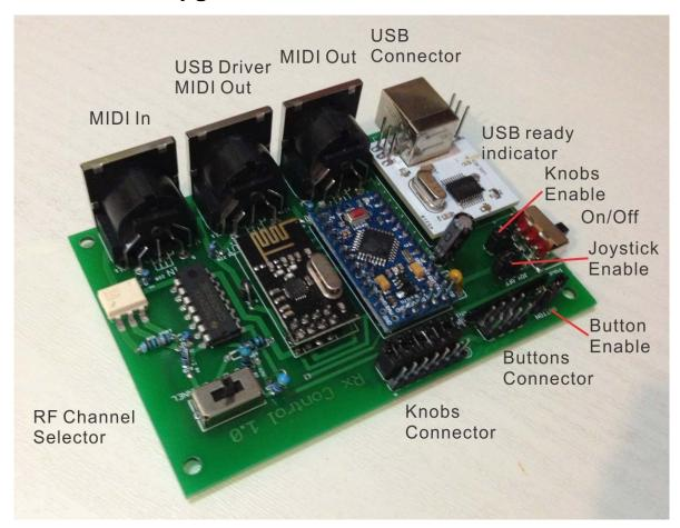
OCTOPUS Rx control is an upgraded version of OCTOPUS receiver which can connect potentiometers(B10K) and buttons to send out realtime MIDI controller messages. You may also use other sensors instead of potentiometer as MIDI control devices.
