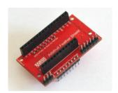
The **Adafruit Feather Shield** is an adapter that allows you to install Adafruit Feather compatible modules in the mikroBUS slot or connect mikroBUS modules (such as <u>MikroElekronika</u>'s Click®) to Adafruit Feather compatible modules.
