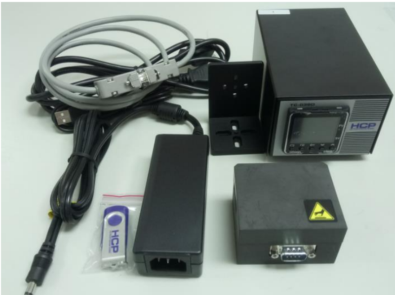
Fig. 1.1.1 TC-038D controller, crystal oven, connection wire and power supply.
