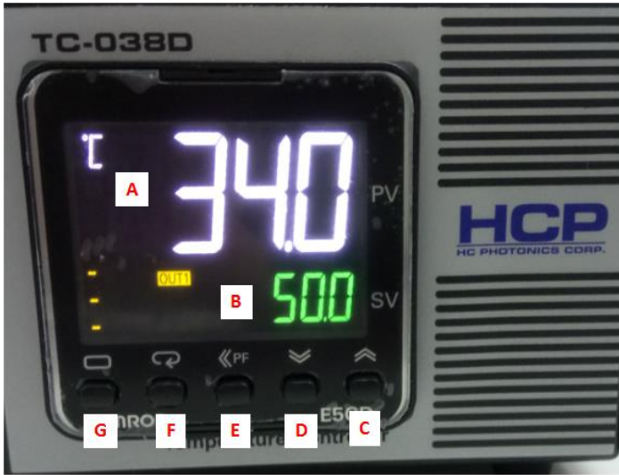
Fig. 1.2.1 The front panel of TC-038D controller, the function of A ~G has been listed in the table below.
