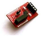
The **BOKRA RS485 Isolated** module is an isolated half-duplex RS485/422 transceiver used as an interface between the UART and the RS485/422 communication bus. The module implements half-duplex communication, has a reliable receiver input, isolation, AutoDirection (automatic direction selection, making the DE and RE signals unnecessary).
