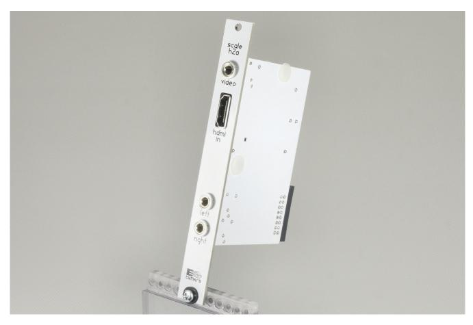
Tymkrs presents the H2A module, a 3hp Eurorack module which converts an HDMI input into left and right line-level audio outputs and a composite video output (PAL/NTSC) via 1/8" jacks.
