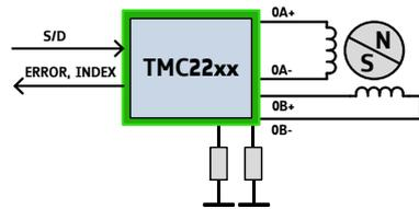
In this example, configuration is hard wired via pins. Software based motion control generates STEP and DIR (direction) signals, INDEX and ERROR signals report back status information.
