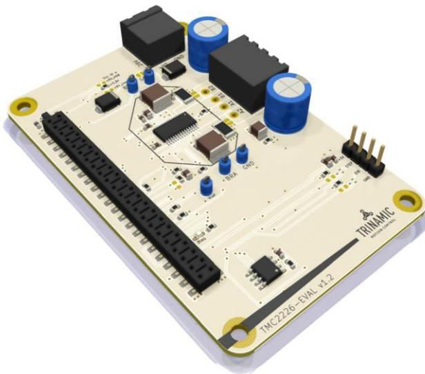
The TMC2226-EVAL is part of TRINAMICs universal evaluation board system which provides a convenient handling of the hardware as well as a user-friendly software tool for evaluation. The TMC2226 evaluation board system consists of three parts: STARTRAMPE (base board), ESELSBRÜCKE (connector board with several test points and stand-alone settings), and TMC2226-EVAL.
