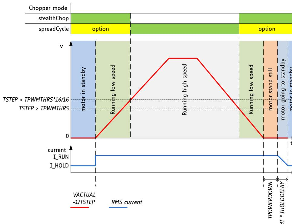
Figure 6.7 TPWMTHRS for optional switching to SpreadCycle
