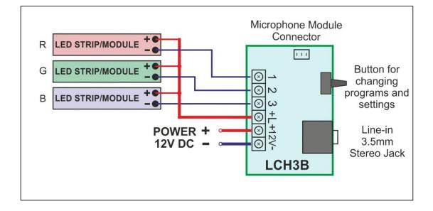
The supply voltage 12VDC is connected to the terminal blocks marked + and - .
