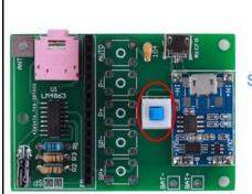
Step 13: Install 1pcs Self-locking Button at S6.
