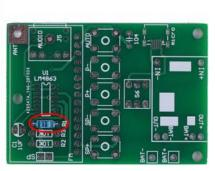
Step 1: Install 1pcs 39Kohm Metal Film Resistor at R1.
