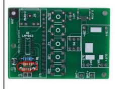
Step 2: Install 2pcs 10Kohm Metal Film Resistor at R2,R3.
