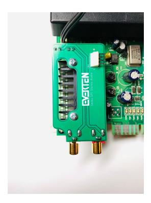
8. Connect the other end of the wire harness to CN1 on the stereo PCB.
