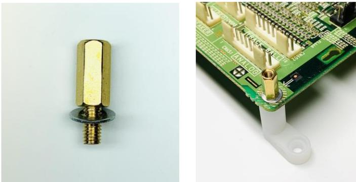
3. It is very important the standoff is securely screwed into the PCB foot. The exposed contacts surrounding the mounting hole provide a ground connection to the stereo PCB.
