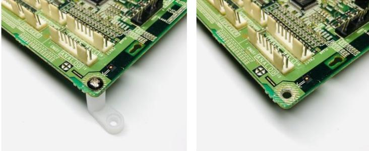
2. Place one of the provided washers on the male threads of the female-male brass standoff. While holding the PCB foot under the mounting hole, firmly screw the standoff into the PCB foot.
