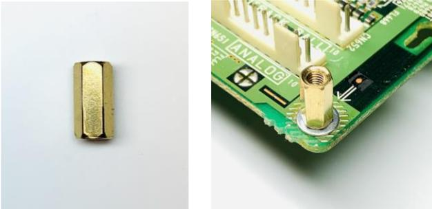
4. It is very important the standoff is securely screwed down. The exposed contacts surrounding the mounting hole provide a ground connection to the stereo PCB.
