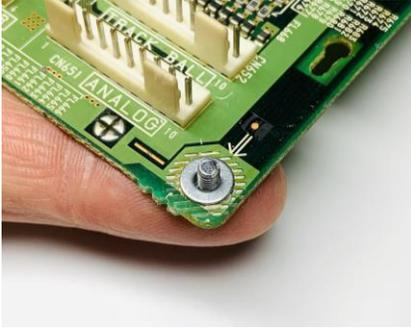
3. Firmly screw the female-female brass standoff on to the exposed screw threads, using a screwdriver if necessary.
