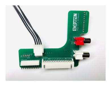
4. Connect the IO board to the Sega ST-V board by lining the connectors up with CN25 and CN21 and pressing down slowly, ensuring all header pins line up with the IO receptacles.
