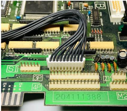
12. For optional spinner switch only; connect the other end of the 3-pin switch harness to JP3 with the exposed contacts facing towards the JAMMA edge. There is no harm in plugging the harness in backwards, it will just reverse the operation of the joystick/spinner switch.
