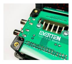
10. Connect the other end of the provided wire harness to the AA connector on the Taito F3 PCB.
