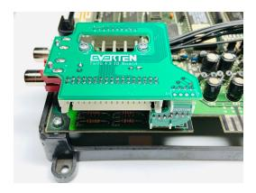
9. For Lions3 case only; as the board lowers into position ensure the stereo PCB is positioned underneath the custom Lions3 left riser screw tabs.
