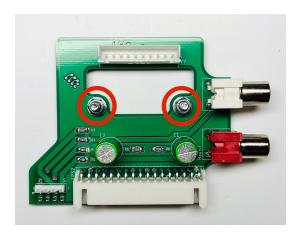
7. Connect the provided wire harness to the AA connector on the stereo PCB.
