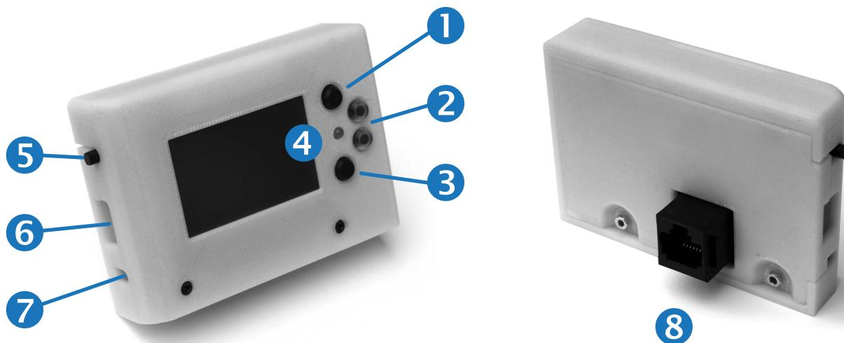
LCD screen and four control buttons are located on front side of the data logger.
