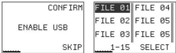
Use UP or DOWN button to scroll through files list. Pressing and holding UP or DOWN button advances to next few files and if files list exceeds one screen first or last file is selected. This can be used to move to the end or beginning of files list quickly.
