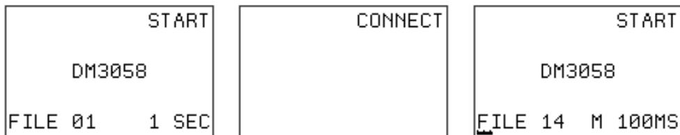
If multimeter was not detected by querying serial commands data logger displays single CONNECT prompt. This is most likely caused by wrong RS232 baud rate setting on multimeter. Connection can be re-checked by pressing START/STOP button.
