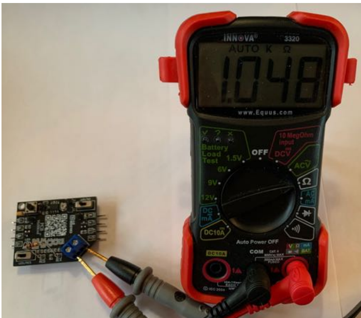
Testing a through-hole resistor.
