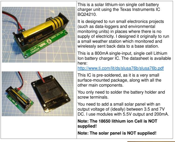
\*Note: We do NOT supply the 18650 size lithium ion cell. This is due to shipping restrictions. These cells are usually available locally.
