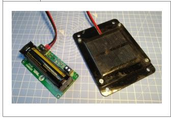
Add a small solar panel wired to the solar input.
