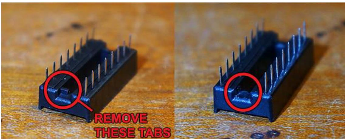
Now solder the socket onto the board on the other side to the header pins, in the position indicated by the silkscreen. The socket solders into the smaller oval solder pads
