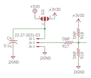
As manufactured, no I/O resistors are populated and none of the supply pins are connected. At the very least, the series resistor position will need to be populated or
