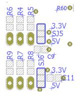
Most external connections to the Teensy are made through three pin connectors, but DIO18 and DIO19 go through a four pin connector and have a slightly different resistor network to accommodate I2C communication and make the pins more flexible.
