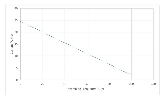
Inverter Continuous Safe Operating Area Ambient Temperature 25°C, DC Bus 36V
