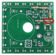
Step 16: Install 1pcs 100Kohm Metal Film Resistor at R5 on Main PCB.
