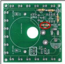
Step 15: Install 1pcs 30Kohm Metal Film Resistor at R6 on Main PCB.
