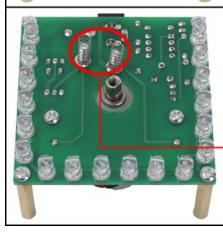
Step 32: Install 2pcs 11\*4\*4mm Metal Spring at 3mm holes. They are used to provide work power for circular rotating PCB.
