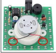
Step 28: Install 1pcs DC3V-9V JS-30 DC Motor at motor. It is a DC motor, so there is no need to distinguish between positive and negative.
