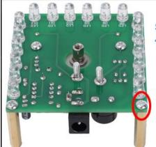
Step 31: Install 4pcs M3+25mm Copper Pillar and 4pcs M3+6mm Screw on Main PCB as a stand.
