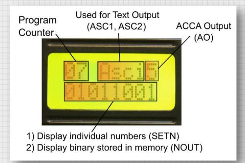
The Program Counter is always displayed on the first two spaces on the first line. The other locations of output are shown above. Note that only output you program will be seen on the display. When a program is run, the display is initially cleared.
