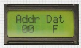
"Addr" stands for Address. This displays the current value of the program counter which will point to the current memory location you are at. When you enter a number from the keypad and press INCR, that value will be stored in memory and the program counter will be incremented.
