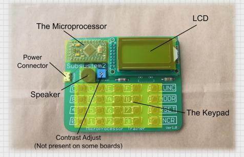
**The Microprocessor**: This is the heart of the computer. It has all of the computing, processing, and input/output interfaces needed to run programs.
