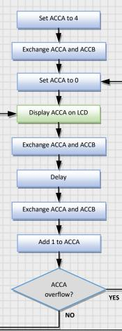
the delay value into ACCA. We then call the delay routine and the exchange ACCA and ACCB again to restore ACCA to the current count. We add 1 to ACCA and look to see if there is an overflow (ACCA>15). If there is none, loop back and display the new number. If there is an overflow, loop back to where we set ACCA to 0 so we can start the count again from there. Let's convert this flow chart to a program.
