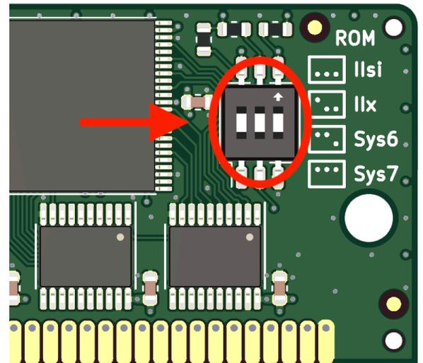
On Macintosh II-series machines, the ROM SIMM socket is accessible by just removing the computer’s top cover. On Macintosh SE/30 machines, the computer must be disassembled and the motherboard removed in order to install the SIMM. Depending on your machine, a jumper may need to be installed or removed to enable the ROM disk.
