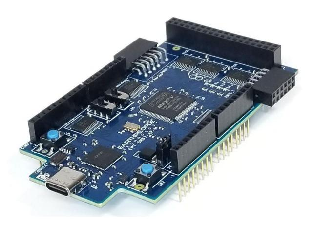
The MegaProLogic is a part of the EPT USB/PLD development system. It provides an innovative method of developing and debugging the users microcontroller code. It can also provide a high speed data transfer mechanism between microcontroller and Host PC.
