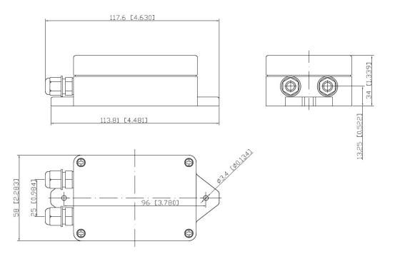
Pic. 2. qBoxMini Enclosure Kit (No SMA) dimensions
