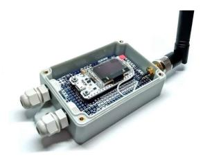
Pic. 17. WiFi LoRa controller with OLED
