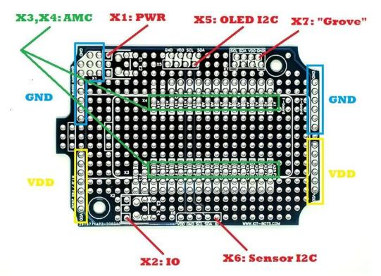
Pic.11. Connectors placement proposal: Arduino MKR Compatible board based
