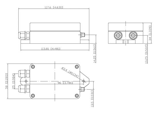
Pic. 4. qBoxMini Enclosure Kit (One SMA) dimensions
