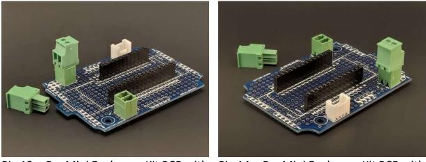
Pic.13. gBoxMini Enclosure Kit PCB with Pic.14. gBoxMini Enclosure Kit PCB with connectors setup for Adafruit Feather connectors setup for Adafruit for Compatible board
