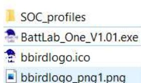
**NOTE:** The SOC\_profiles folder **must** be present and contain the State of Charge (SOC) .csv files for the batteries you intend to use. Bluebird Labs will be updating these from time to time so please check the website for newer profiles at [www.bluebird-labs.com](http://www.bluebird-labs.com).
