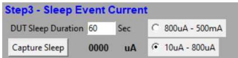
**NOTE:** If you do not know your expected range, select the 800uA – 500mA range. If the actual sleep current falls below this range then Battlab-One will pop up a message and recommend the **10uA-800uA** range. **Selecting the 10uA-800uA range may damage the Battlab-One shunt resistor if the power output of your sleep mode state is greater than 1 Watt (e.g 4.5 volt PSU output x 225mA sleep current = 1.01 watts).**
