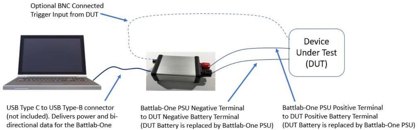
Figure 2. System Connections
