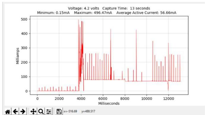
**Sleep Capture Duration:** This allows the user to select the duration that Battlab-One will use to average the captured current in Step 3.3 above.
