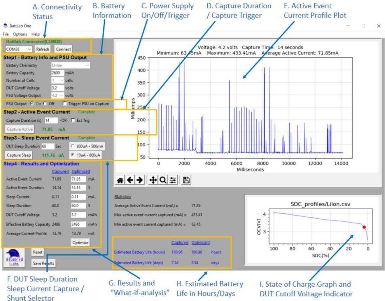
Figure 1. Battlab-One Application Software
