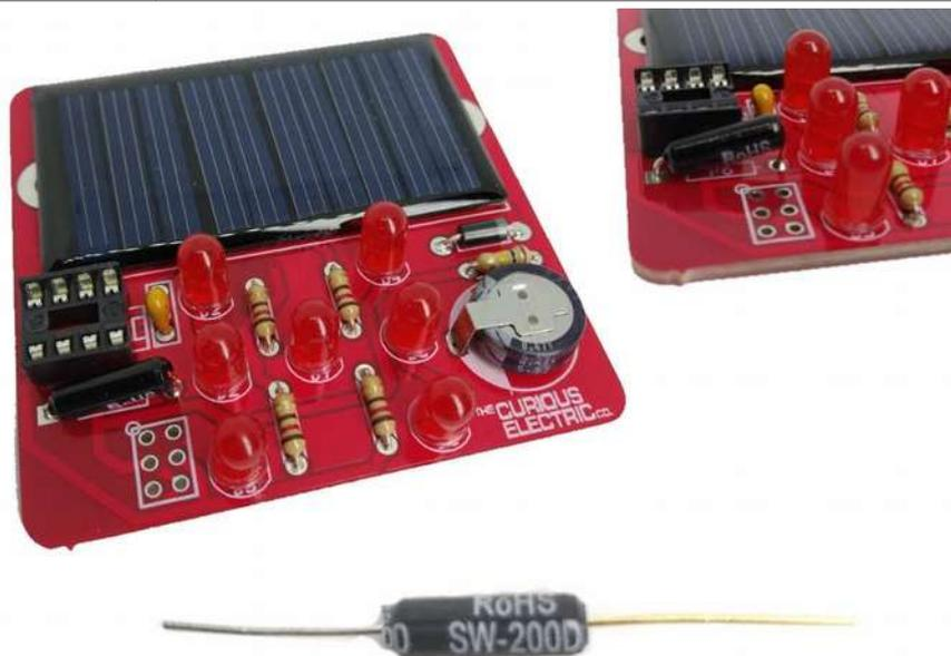
The vibration switch contains a small metal ball which connects some contacts to trigger the circuit.
