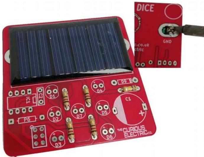
The solar panel must be soldered with the correct orientation. The solar panel has a + and a – marked side, which must align + to + and – to GND on the PCB.
