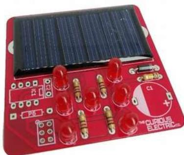
Ensure correct orientation for D9, the 1N5819 diode. This has tiny markings saying “1N5819” and also a white band around one end to indicate polarity. Ensure the white band on the diode aligns with the white band marked on the PCB.
