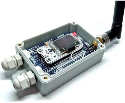
Pic. 17. WiFi LoRa controller with OLED
