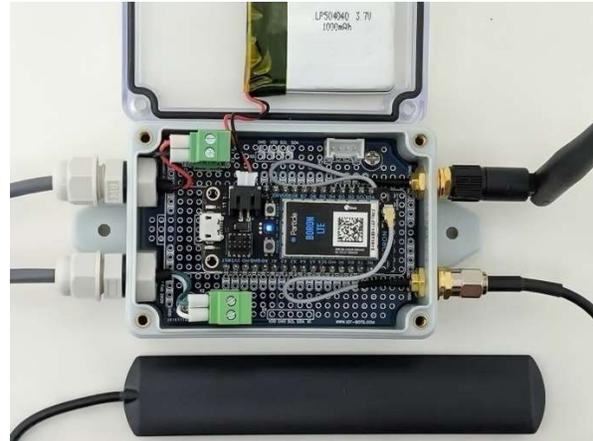
Pic. 16. LiPol battery applied to a transparent lid (inside view)
