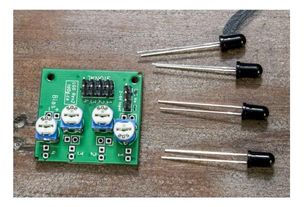
The photodiode are oriented with the anode (longer lead) adjacent to the edge and the cathode (shorter lead) next to the potentiometers. A simple way to install the photodiodes in a difficult location (such as the DIY ballistic chronograph) is to insert the photodiode and bend one of the leads over.
