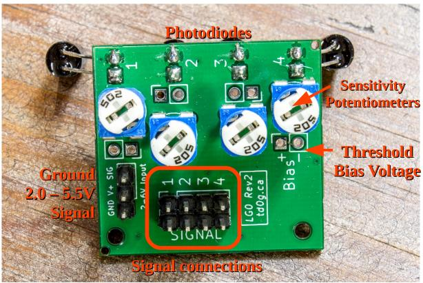
Connecting to the LG0 Light Gate sensor is simple. Connect a power supply to the GND and V+ pins, then connect the SIG pin to your microcontroller.
