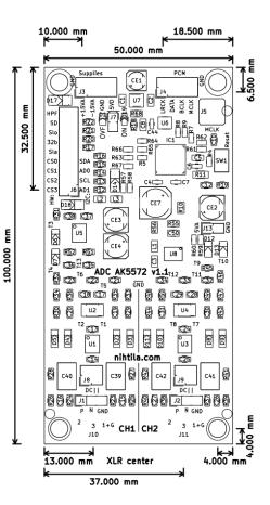
Master clock (MCLK) can be brought to PCM pinheader J4, or optional SMB connector J5 and 50  $\Omega$  resistor R11 can be populated.
