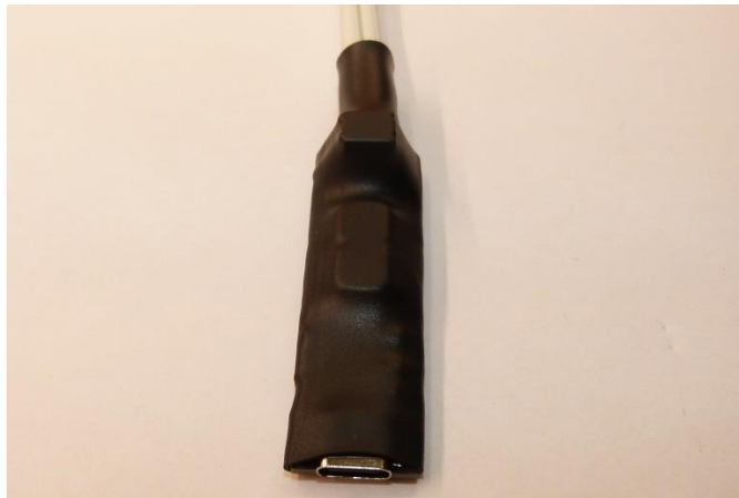
Figure 11: Finish shrinking at the cable end.
