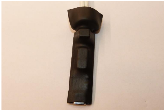
Figure 10: To add more strain relieve, add thinner heatshrink on the wire before inserting into the terminal block.
