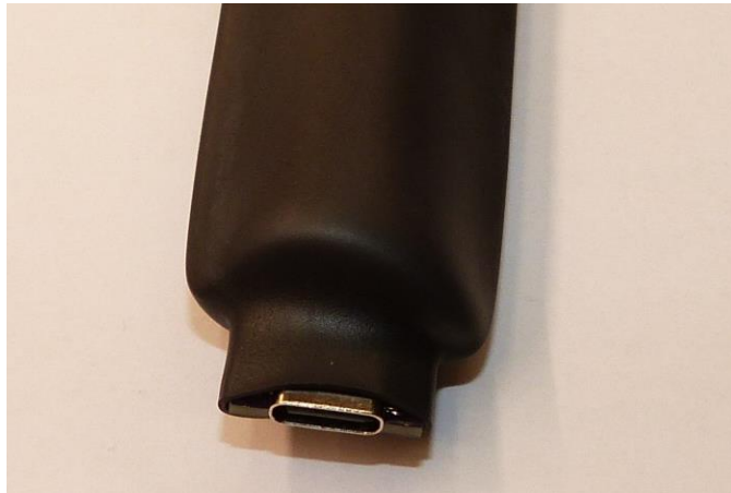
Figure 8: Work the hot air along the tube from the USB connector to the wire end.
