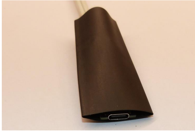
Figure 7: Start heatshrinking at the USB-C connector end.
