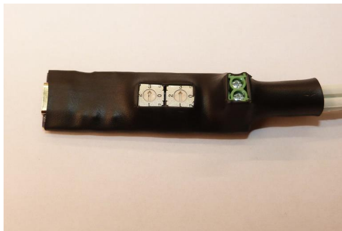
Figure 12: If you forgot to set the switches or want to change them, the topography of the heatshrunk board lets you pick cutouts for the switches or terminal block easily.
