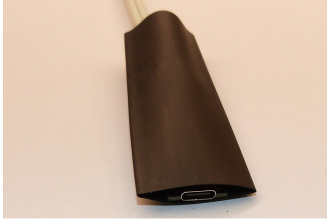
Figure 4: Start heatshrinking at the USB-C connector end.
