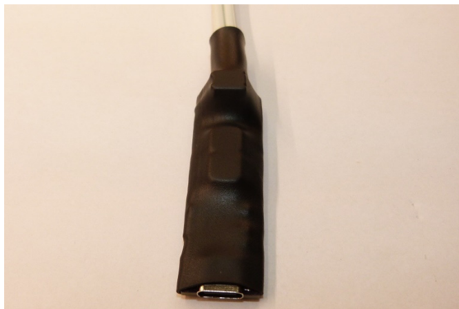
Figure 8: Finish shrinking at the cable end.
