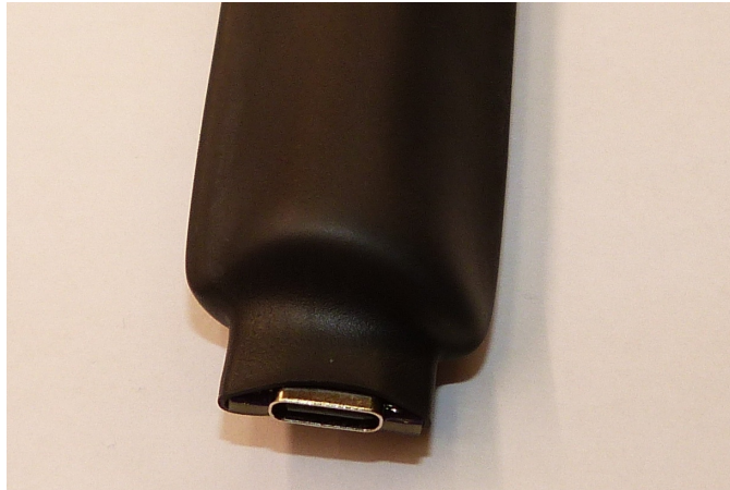
Figure 5: Work the hot air along the tube from the USB connector to the wire end.
