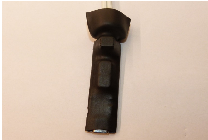
Figure 7: To add more strain relieve, add thinner heatshrink on the wire before inserting into the terminal block.
