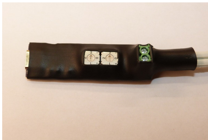
Figure 9: If you forgot to set the switches or want to change them, the topography of the heatshranked board lets you pick cutouts for the switches or terminal block easily.
