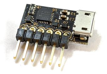
It features the Silicon Labs CP2102N chip for excellent cross platform driver support, on-board autoprogram circuitry to transparently handle device programming and serial console use, a V+ blocking diode and ESD protection.
