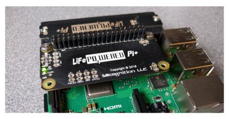
External power has to be connected to the LiFePO<sub>4</sub>wered/Pi+<sup>TM</sup> instead of the Raspberry Pi's own power input. This is necessary to allow battery charging and to ensure that the LiFePO<sub>4</sub>wered/Pi+<sup>TM</sup> has complete control over the Raspberry Pi's power.
