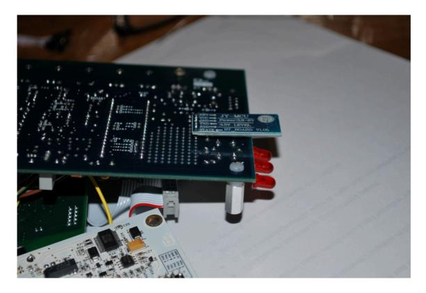
**If you have an MS3 cpu**, remove the MAX232 serial chip. Serial is not needed because MS3 has USB. Solder 4 wires in the empty locations in pin 11, 12, 15 and 16 (see pic below).
