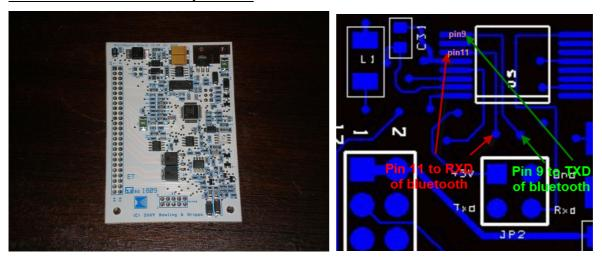
The MSPNP / DIYPNP have a white (MS2 based) microsquirt module in them. The serial chip is located on the top left corner of the board (see picture above). It has the number MAX3221 on it and has 16 legs. The chip is a lot smaller than the one used in the regular megasquirt, so be careful when soldering wires to it
