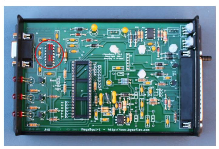
The V2.2 board has no proto area, so you need to use hot glue to install the module.
