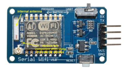
**IMPORTANT**: If you have a WiFi module with the optional **external antenna**, you must remove the component (it's a jumper actually) next to the antenna connector (see pic above). Carefully pry it off with a small screwdriver, no need to desolder. It comes off very easy. If you do not remove it, the external antenna will not be activated. If you bought the module + antenna from me, I have already removed the jumper for you ©.
